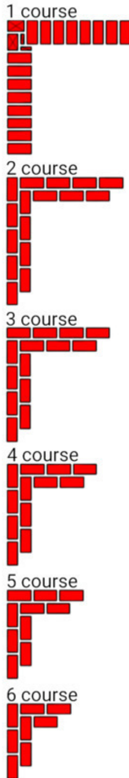
Fig.3. The order of laying bricks in the corner of the walls. Wall thickness 1 brick.
