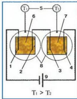
1—4. electrodes made of stainless steel
