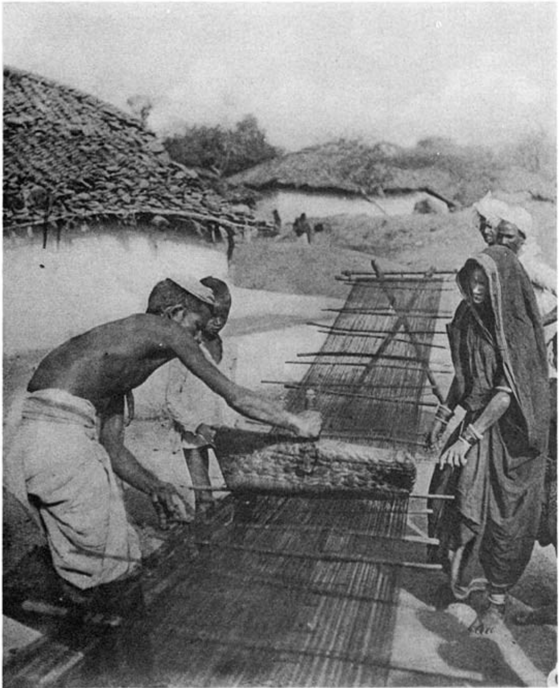
Weaving: sizing the warp
