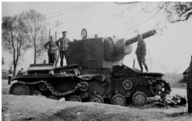
German military inspect the Soviet tank KV-2 with a broken chassis. Even without enemy shells, the heavily loaded chassis of the KV-1 and KV-2 tanks often fail
