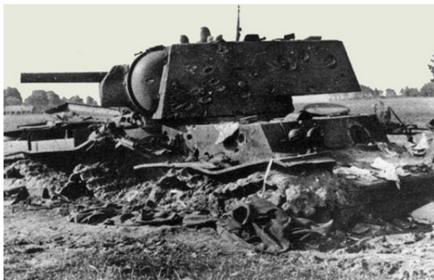
The Soviet tank KV-1, smashed by dozens of hits. July 1941, the south of the USSR. Armament: 76 mm. gun, 90—114 shells, three 7.62 DT machine guns (course, paired with a gun, aft). Booking: the forehead, the side of the hull is 75 mm., The forehead, the side of the tower is 75 mm. (protection from an armor-piercing shell of a 50-mm German cannon further 200 meters). Crew of 5 people. Weight 48 tons. Common problems with the transmission. Speed on the highway 34 km. h, the reserve for cross-country terrain is 120 km. Specific power 11.6 hp, ground pressure 0.77 kg. see From 1939 to 1942 produced 2770 machines.
